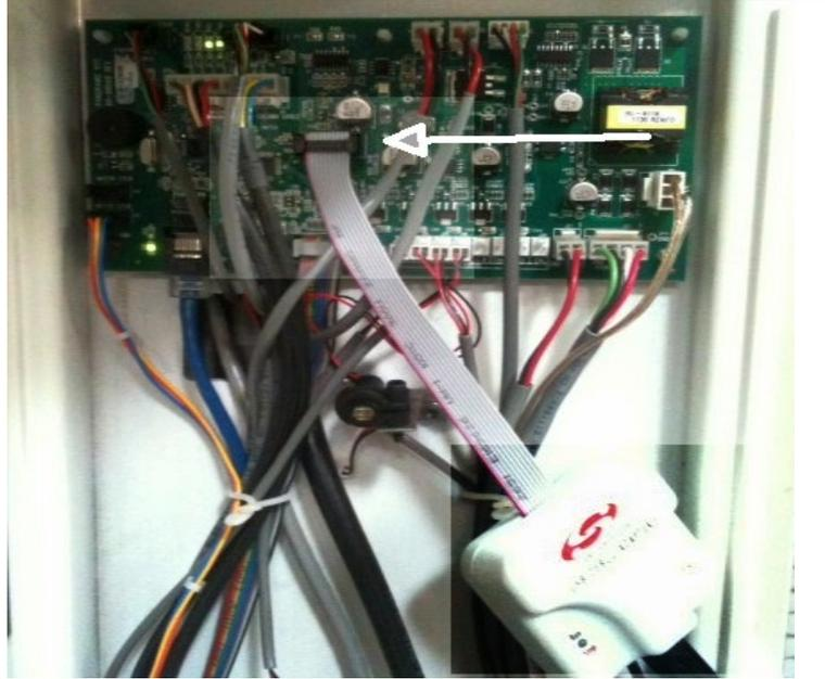
14. Connect the other end of the **USB DEBUG ADAPTER** (USB Cable) to an available USB port on the **Vantage PC**.
